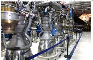
of thrust at liftoff, rising to 716 kilonewtons (161,000 pounds) as it climbs out of Earth's atmosphere. Merlin's thrust-to-weight ratio exceeds 150, making the Merlin the most efficient booster engine ever built, while still maintaining the structural and thermal safety margins needed to carry astronauts.
