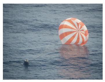
SpaceX will use a 150-foot boat equipped with an A-frame crane and two inflatable boats to perform recovery operations. On board will be approximately a dozen SpaceX engineers and technicians as well as a four-person dive team. Once Dragon splashes down, the team will first secure the vehicle and then place it on deck for the journey back to shore.
